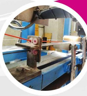
Multi-core cables are made with the best twisting step in order to ensure the best flexibility.
